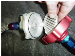
An 8-micron filter on a dry-break arrangement makes for easy servicing.
